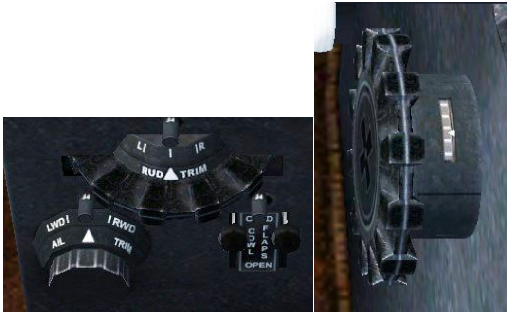
Rudder and aileron trim controls and indicators (left) and elevator trim control and indicator (right)
